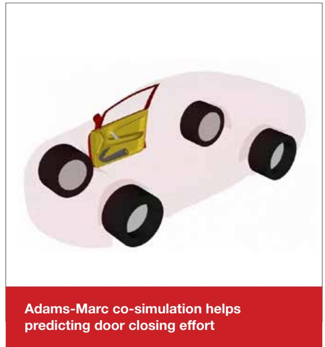
**“Throughout the co-simulation, the dynamic behavior of the door is calculated by MSC Adams and resistance of the seal is calculated by MSC Marc. The accurate results of the co-simulation were provided to our customer and helped win the order to supply seals for a new model vehicle.”**
